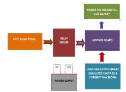
Figure 6: Block Diagram APFC
