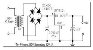
Figure 7: Power Supply System
