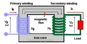
Figure 17: Working Principle of Transformer [16]
